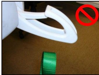
Figure 13E - Sling loop separated from the P-600 carry bar hook.
