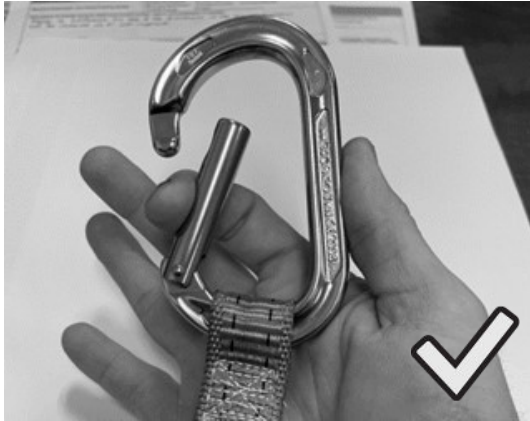
Figure 8A: Correct orientation
