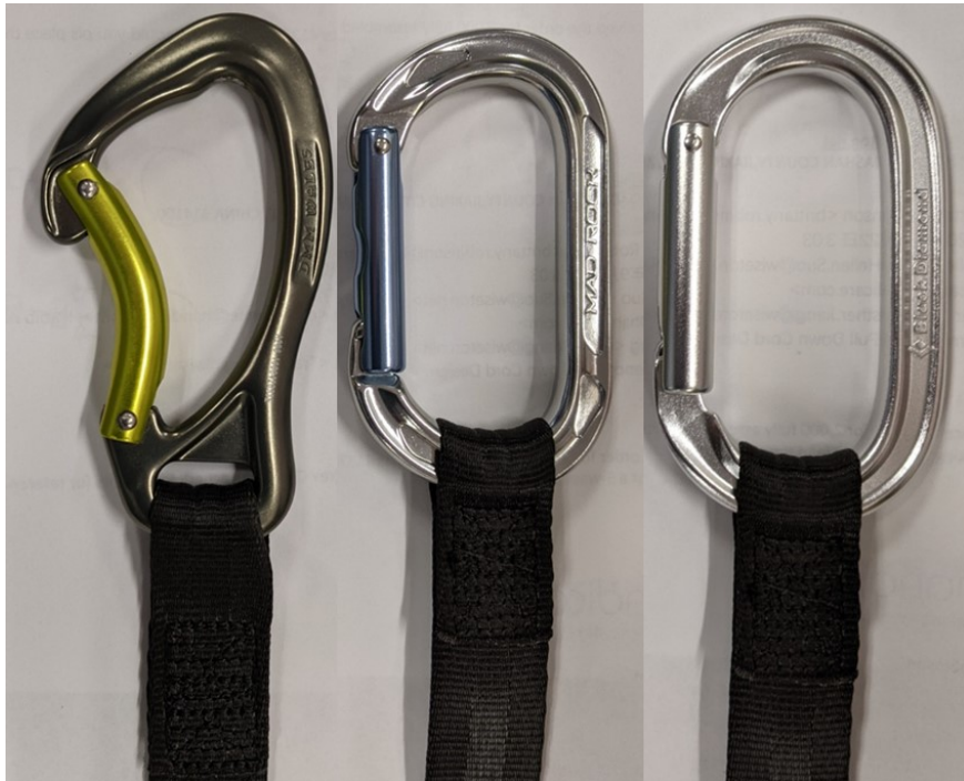
Figure 8C: Various carabiner styles used in P-440
