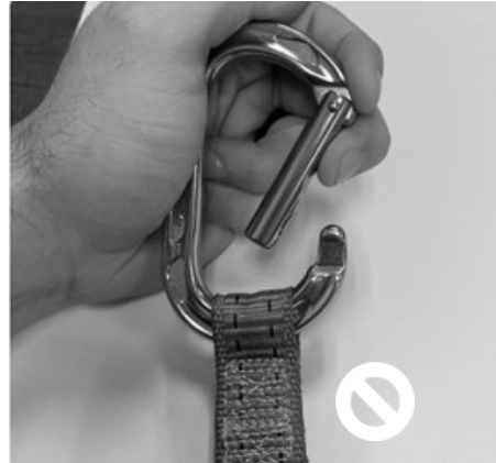
Figure 8B: Incorrect orientation
