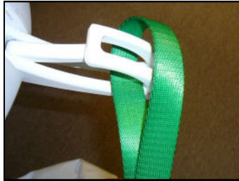
Figure 13B - During the preparation for the patient transfer, the sling loop flipped
