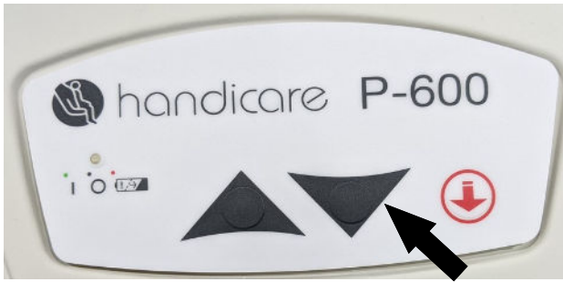
Figure 15A –Lift showing DOWN button located on front right side of lift.
