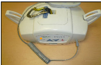
Figure 14E - Charger is connected to the lift. The indicator light on the charger will be ORANGE indicating that the lift is charging.
