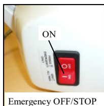
Figure 15D - Close-up of switch ON - Normal lift Operation OFF - Emergency Stop
