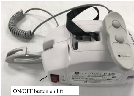
Figure 15C –RED Emergency stop switch located on the front left side of the lift.
