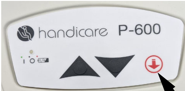
Figure 15B –RED emergency lowering button located on middle of the front of the lift.
