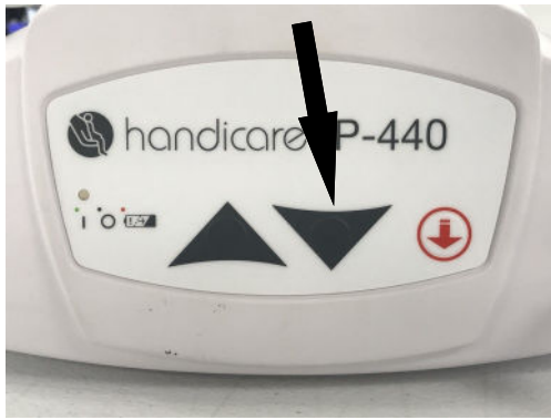
Figure 15A –Lift showing DOWN button located on front right side of lift.
