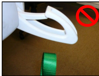
Figure 13E - Sling loop separated from the P-440 carry bar hook.
