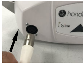
Figure 14D - Connect the charger to the lift. Be sure to line up the 3 metal prongs on the end of the charger with the 3 holes in the black lift "DC" connection.
