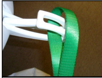
Figure 13B - During the preparation for the patient transfer, the sling loop flipped
