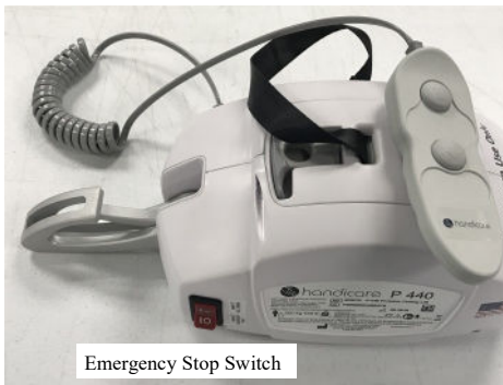
Figure 15C –RED Emergency stop switch located on the front left side of the lift.
