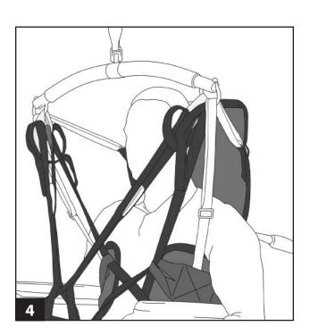
Attach both the legs and thoracic straps to the lifter using the appropriate color coded loops. With the arms on the outside (through the counterbalance strap) attach the strap to the lifter.
