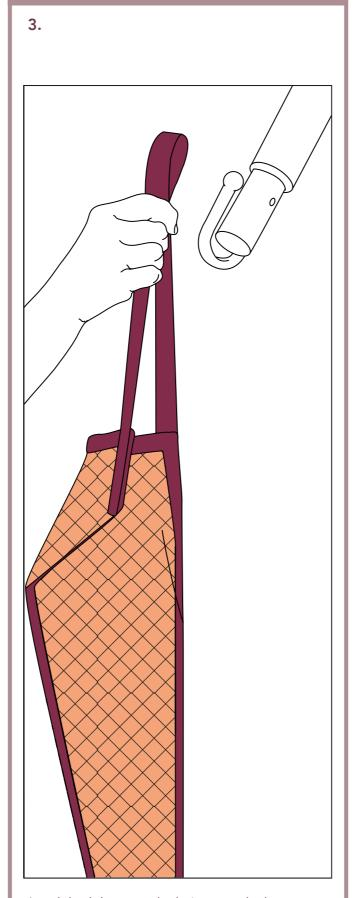
Attach both loops to the hoist spreader bar.
