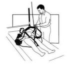
4. Attach sling's leg and back straps to carry bar for desired sling inclination. See instructions for various inclination positions.
