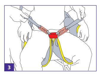
Glide each leg section under each thigh. Ensure that the leg sections are not twisted. Connect leg straps together by taking the right leg strap and thread through the modesty loop.
