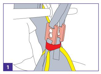
With the leg straps threaded through the modesty strap, attach clips to the lower stud on the spreader bar. When securing the clips there should be a click sound to confirm the clip is located correctly.
