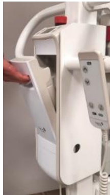
Image 3: Disconnect the NORA Pro from the power supply by activating the emergency stop button. Remove the battery as described in chapter 13.6.1.
