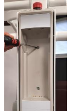
Image 6: Loosen and remove the screws with cross-head screwdriver (PH1).
