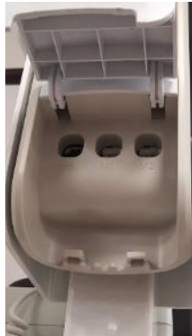
Image 6: Loosen and remove the screws with cross-head screwdriver (PH1).
