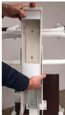
Image 7: Pull the control unit upwards out of the holder.
