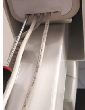
Image 4: Open the connection flap and disconnect all plug connections from the control unit: - Hand control - Lifting motor - Spreader motor - Charging plug, if applicable.
