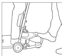
Adjust the lower-leg support so that the upper edge of the plate is about 3 cm/two fingers below the lower edge of the kneecaps. Pull the two pins to loosen. Adjust to the appropriate height.
