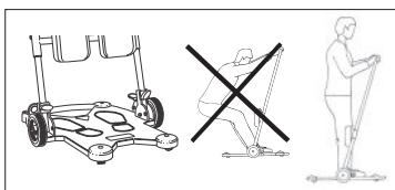
The feet are placed one on either side, see foot markings on base plate.
