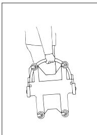
The chassis and raising ladder can be carried separately. Carry the chassis by holding the tube on the front end of the product.
