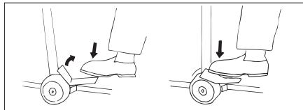
There is a brake for each wheel. With your foot, press down on the red marking on the brake plate. Press all the way down.
