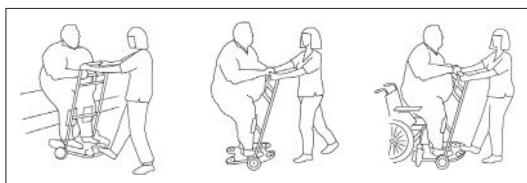
Remove/raise the wheelchair foot plates, and then run the ReTurn in towards the wheelchair. The user places his/her feet on the foot plate, grasps the raising ladder, leans forward, and then lifts from the seat. The caregiver provides counter pressure. Slide the user farther back in the chair when he/she has lifted slightly from the seat.
