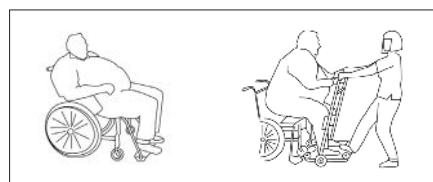
If the user slides forward in the wheelchair, the ReTurn can be used to help the user to slide farther back in the chair.
