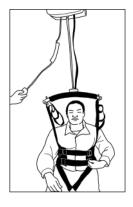
3. The straps can be attached to the carry bar. We recommend the first loop be used as an initial starting point. The straps should bear the same weight distribution on each side.
