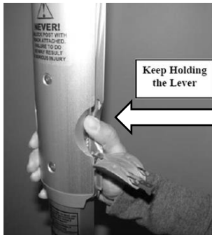
Figure 36: Release Pressure from the Ratchet
