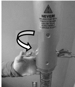
Figure 15: Open the Post Level Fully
