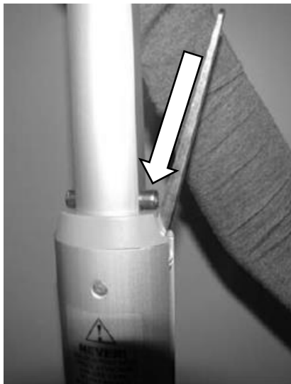
Figure 41: Bottom Pin Touches the Plastic Cover
