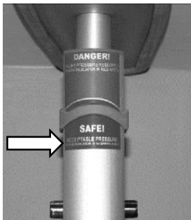
Figure 19: Pressure Gauge in the Safe Zone
