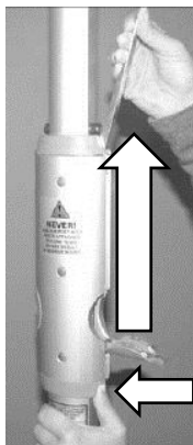
Figure 13: Engage the Magnet
