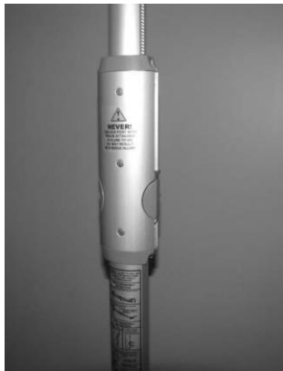
Figure 21: Safety Lock and Level Engaged
