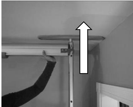
Figure 33: Lift Up to Unhook the Track
