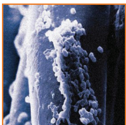
Microbe growth on untreated strap fibers
