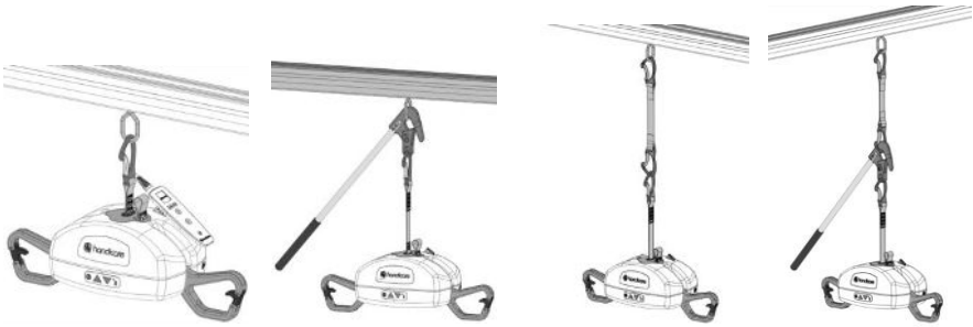
Figure 9: Left to Right - Standard Connection | Reacher Arm Connection Lanyard Connection | Reacher arm and Lanyard Connection.
