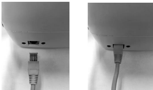
Figure 3: Hand Control connector with latch being inserted into lift connector
