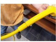
Picture 3: Unscrew the unit screw from the disinfectant hose.
