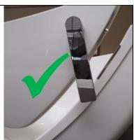
The picture shows the door in the end position; the door can now be locked with the handle.
