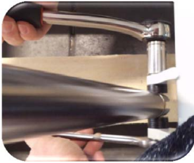
Picture 9: Loosen and remove the lock nut on one side of the shaft.
