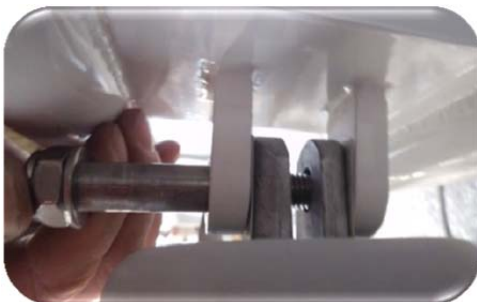
Picture 15: Remove the shaft on the underside of the motor.
