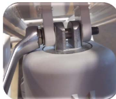
Picture 14: The picture shows the upper shaft with the lock nut removed.
