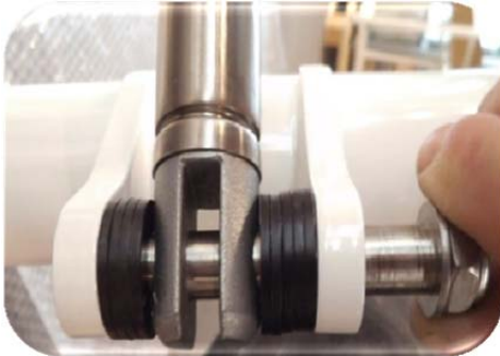
Picture 11: Remove the shaft on the spindle of the motor.
