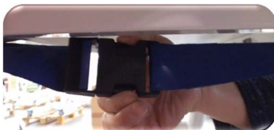
Picture 1: As shown here in the picture, actuate the 1st quick release fastener on the underside of the SINA shower trolley.
